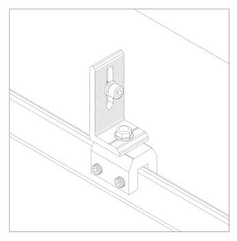
2. Tighten the L foot connector to 15 N·m using 6 mm Allen key or hex driver bit
