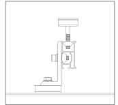
2. Place second PV module into rail, leaving a 20mm gap between modules and insert the mid clamps, slide the PV module flush against mid clamp closely, then tighten the mid clamp screw to 10 N·m using 6 mm Allen key or hex driver bit. Repeat procedure for follow mid clamps.
