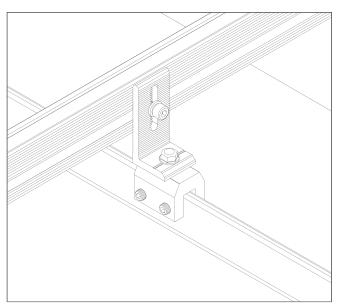
3. Connect rails to L foot to 16 N·m using a M6 Allen key or hex driver bit
